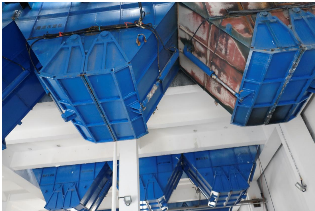
压滤厂房一层接料漏斗
